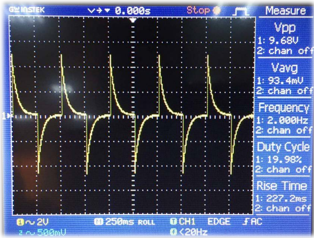
Fig.(4.2) :Reading of out put carry binary counter (4060)IC
